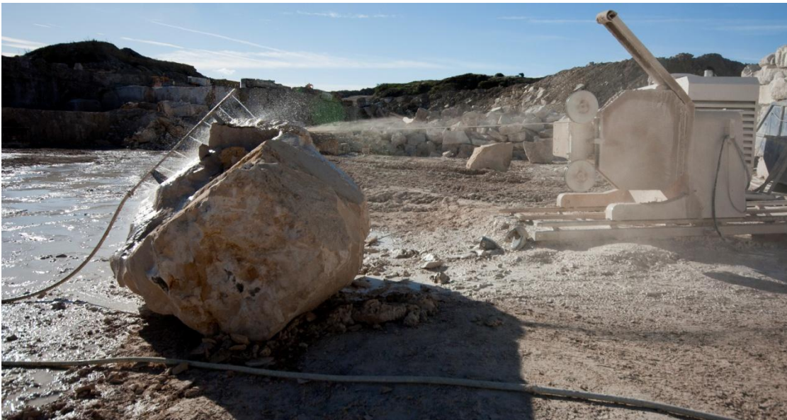
Fig. 13. A Fantini, poly-crystalline diamond tipped chain-saw mounted onto a JCB tractor, squaring blocks in Bowers Quarry.
