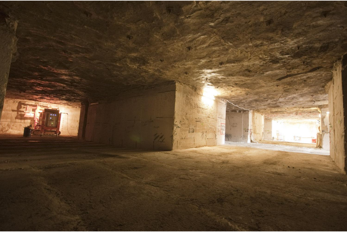
Fig. 16. Jordans Mine is designed with a 75% maximum aerial extraction ratio, with roadways and pillars set out on an approximate 6m x 6m grid.
