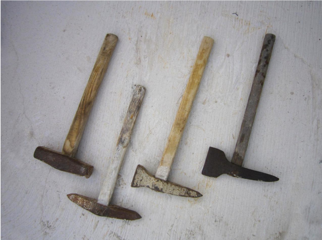
Fig. 8. Traditional Portland quarryman’s hand tools used to extract and “square” blocks of stone (left to right); Sledgehammer, twibel, kivel and axe.
