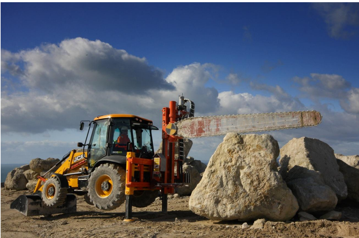
Fig. 13. A Fantini, poly-crystalline diamond tipped chain-saw mounted onto a JCB tractor, squaring blocks in Bowers Quarry.
