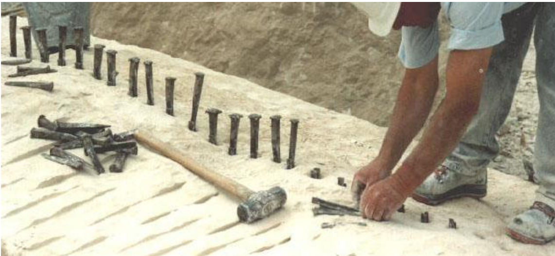
Fig. 9. Plugs & Feathers, a now largely out-dated method used to cut a quarry blocks by exerting a tensile stress into stone, eventually inducing a linear fracture.
