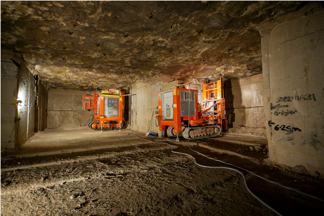
Fig. 15. TwoFantini GU50 mining machines cutting Roach and Whitbed in Jordans Mine.
