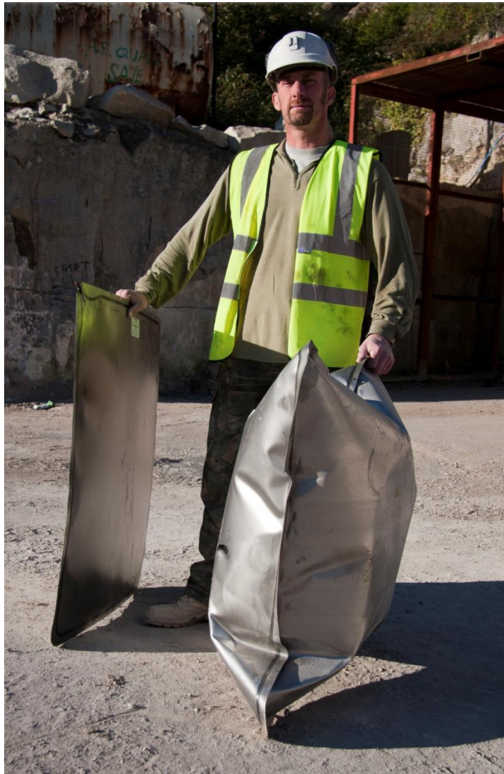
Fig. 11. 1m 2 high tensile steel Hydro-bags, only a few millimeters thick when empty (left), can be inserted into cuts to displace stone through several hundred millimeters (right) by producing forces equivalent to many hundreds of tonnes when slowly inflated with pressurized water. When using Hydro-bags, it is usual to inflate several (evenly spaced along a cut) simultaneously.
