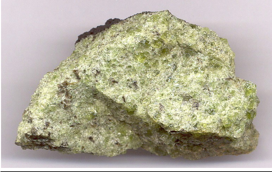
Fig. 1. Hand specimen of a dunite nodule from Lanzarote. Note the pale olive-green colour of the fresh, unweathered, gem-quality olivine. Specimen is 10 cm long.
