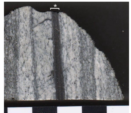
Fig.1. Thin pseudotachylite vein (asterisked) in a banded gneiss specimen from the Reisseck Group, Austria. Note offshoots. Scale intervals: cm. Photo: Giles Droop.
